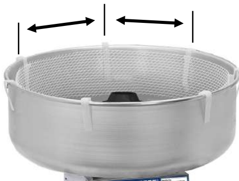
Step 4: Repeat for all clips keeping equal spacing around pan (number of clips varies by model). Allow air space between pan and screening for proper operation.
